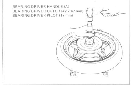
Install the bearing retainer and punch it.
