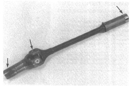
Drive out the spring pin. Separate the drive shaft joint from the drive shaft.
