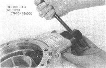
BEARING RETAINER B OIL SEAL, O-RING REPLACEMENT
