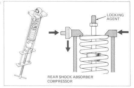
Apply locking agent to the rod threads. Place the upper joint in a vise and tighten the rock nut securely.
