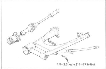
Install the right pivot in the bearing inner.
