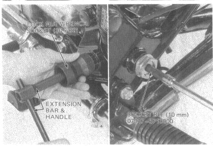
Free the drain tube, etc. from the clamps. Remove the right pivot.
