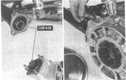
Apply lithium-based multipurpose grease to the splines of the rear wheel and ring gear shaft. Insert the distance collar into the ring gear shaft in the direction shown.
