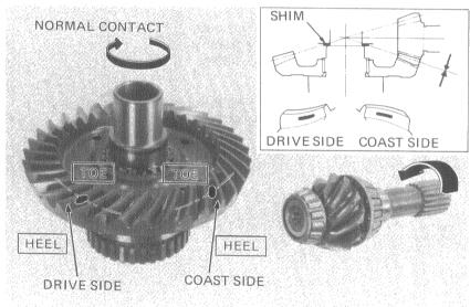
Replace the ring gear shim, if the patterns are not correct.
