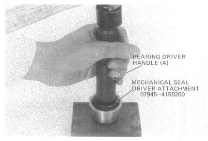
Install the bearing holder so that the flange is seated against the frame body.
