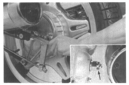
Loosen the axle holder bolt.
