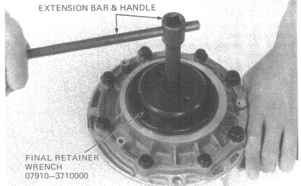
Separate the left case cover from the ring gear and bearing.
