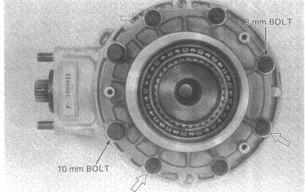
Install the preload retainer A with the oil seal and O-ring assembled in the retainer.
