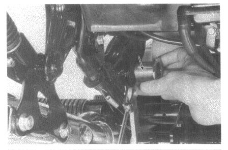
Install the brake torque link on the swing arm. Insert the propeller shaft through the swing arm and install the boot.
