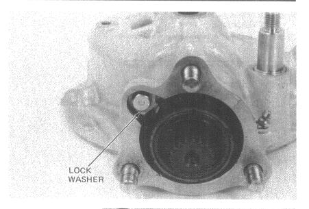
Remove the bearing retainer B.
