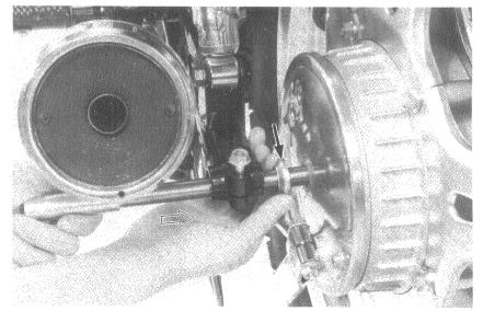
Torque the final gear case to the swing arm and shock absorber mounting nut.
