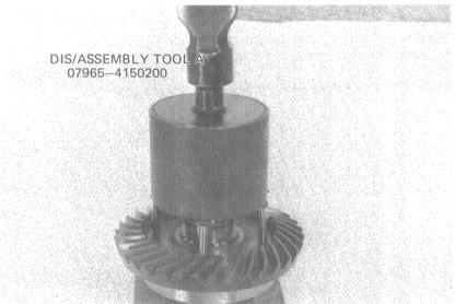
Install the ring gear bearing on the ring gear.
