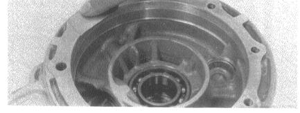
Clean the cover mating surface of the gear case with an oil stone.
