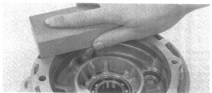
Apply liquid sealant to the mating surfaces of the gear case and cover.
